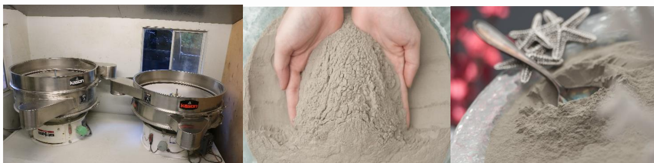
Organic material, sand and larger particles are all screened out to produce an Ultra-fine Clay
