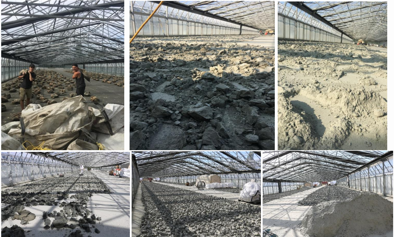
Unpacking burlap sacs Clumps are slowly reduced to a fine powder using our propriety process
